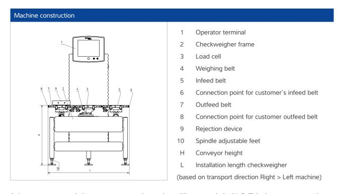
A three-part conveyor belt system transports the products. All conveyor belts (4, 5, 7) in the system run at the same speed to ensure that products are transferred smoothly onto and off of the weighing belt. The weighing process is carried out dynamically and automatically without intervention by operating personnel. The weight value, including mass unit, is converted and shown on the display.
