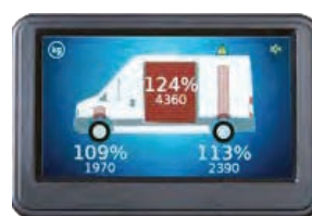
GROSS OVERLOAD WARNING
