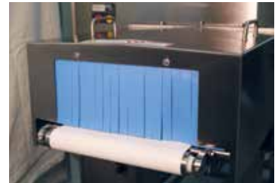
Hygienic design through chamfered surfaces
