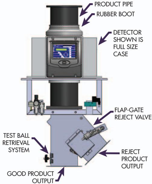
Also... a metal detector can be configured to operate in 'Pipeline' mode, where the product is generally pumped through the system (shown below) and contamination is diverted away from the product flow through the 'Reject Valve'.
